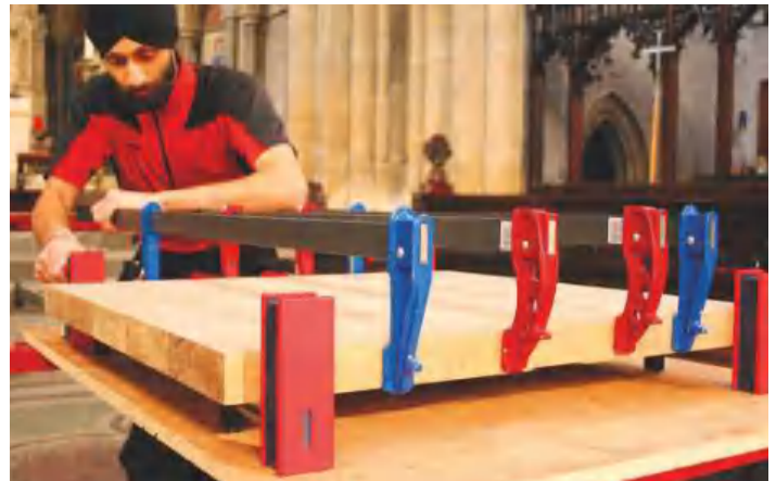
▲ Pic.11 Clamping and screwing everything together to ensure an even pressure
